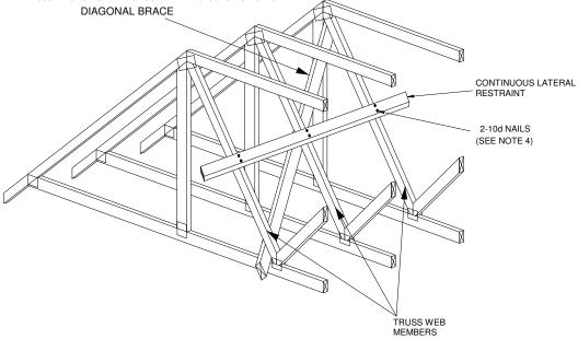
This information is provided as a recommendation to assist in the requirement for permanent bracing of the individual truss web members. Additional bracing may still be required for the stability of the overall roof system. The method shown here is just one method that can be used to provide stability against web buckling. MiTek USA, Inc.
